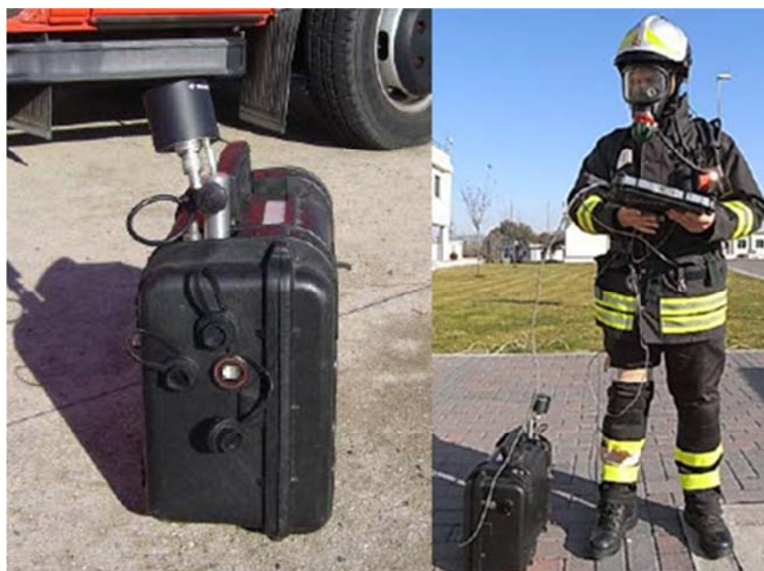
Figura 0-13 - Terminale mobile Access point (AP) - Dropped Unit – Progetto LIAISON
