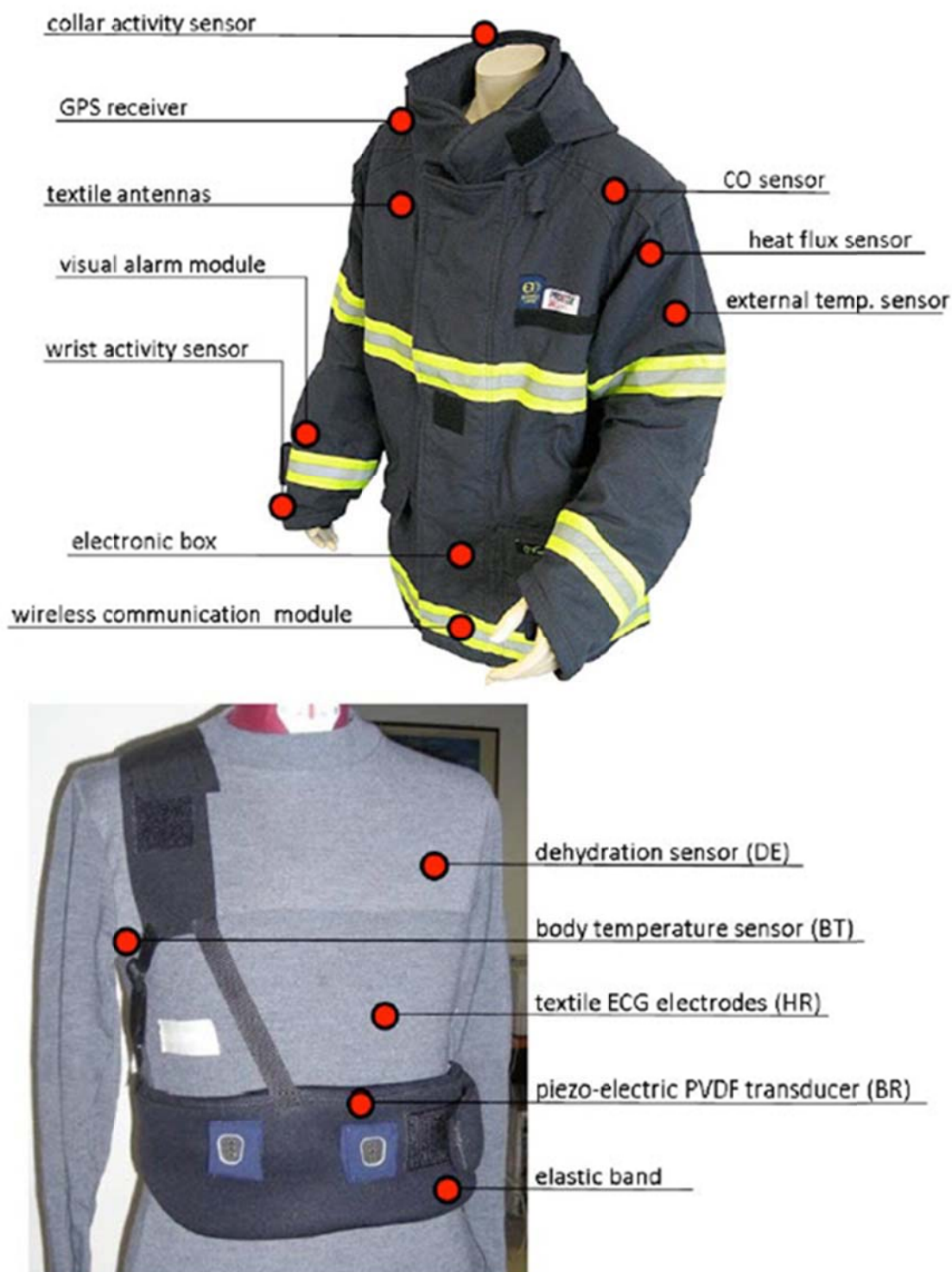
Figura 0-16 - ProeTex (Protection e-Textiles: micro-nano-structured fiber systems for emergency-disaster wear) posizionamento e tipologia dei sensori
