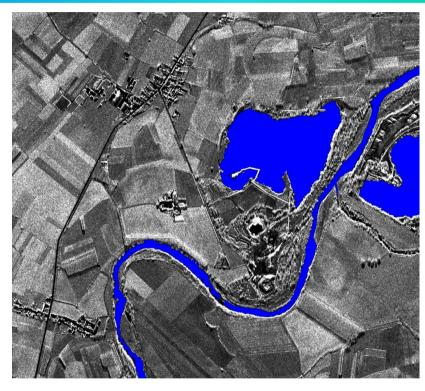
• Water bodies are extracted thanks to a threshold operation over the original SAR image, followed by selective suppression of blobs and smart correction of contours
