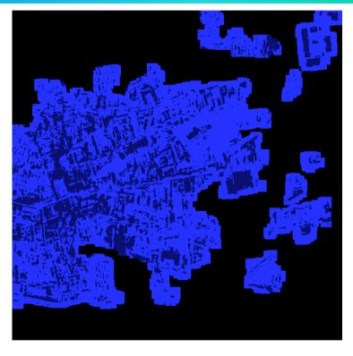
• The extraction of the most significant objects in 3D may be obtained by suitable thresholding of the Digital Building Model, DBM (DSM-DTM) inside the urban area. Because of the "spatial mean" effect of the IfSAR DSM and the slant to ground projection operation, only medium to large structures can be identified.
