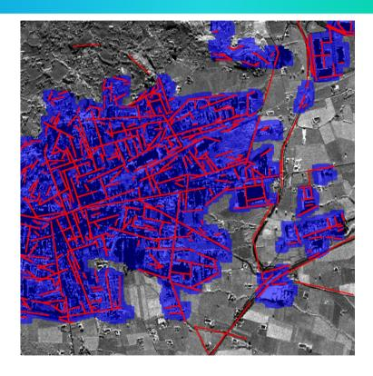
• It is possible to exploit the information on urban street height to improve the road network detection with respect to 2D-only characterization.
