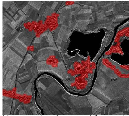
• Clues on the presence of man-made objects are given by textural features in the images, while geometrical constraints in addition to location and orientation help locating them and outlining them precisely.
