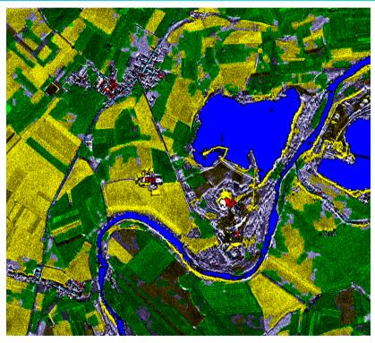
• Classification and segmentation provides a first subdivision of the fields in the rural area according to their backscattering behaviour.
