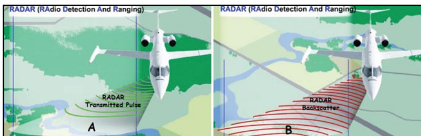
Figure 5-1: Schematic illustrating how radar works.
