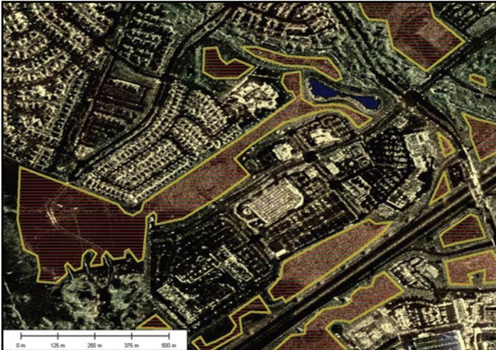
Figure 7-4: Unobstructed regions of modest and constant slope (yellow polygons) are suitable locations to test the data.
