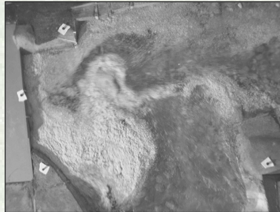
With sawdust to improve the water reflectivity
