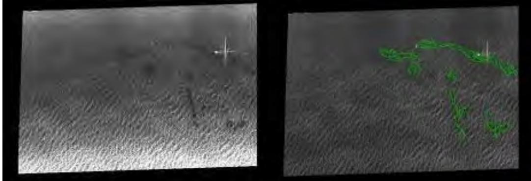
Oil spill and ship detection
